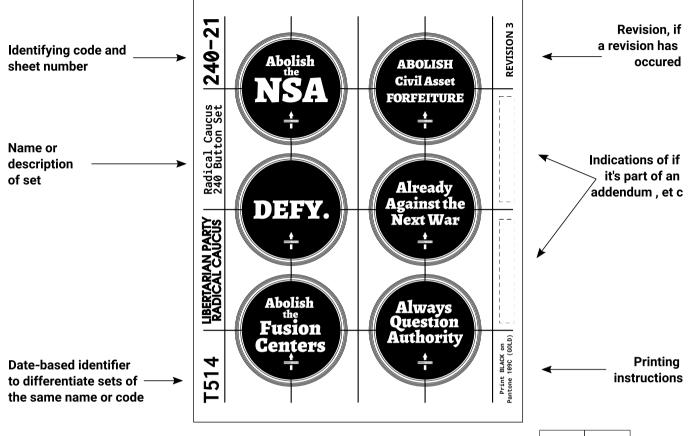
To cut circles with a circular punch, cut into strips along vertical lines between buttons and edges
