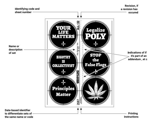
To cut circles with a circular punch, cut into strips along vertical lines between buttons and edges
